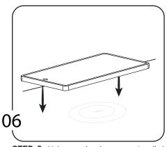
STEP 6: Make sure the charger was installed correctly by placing a wireless charging compatible device in the center of the charger. Check that the device is charging a few seconds after it is placed.
