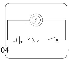
**STEP 4:** Using a 2A fuse, attach wires to a 12v power supply and ensure there is a waterproof connection.
