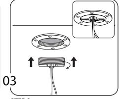
STEP 3: insert the charger into the locknut and turn until it is firmly in place.
