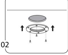
**STEP 2:** Use the provided self tapping screws to attach the locknut to the underside of the charging surface. Next apply 3M 5200 adhesive to the center of the hole.
