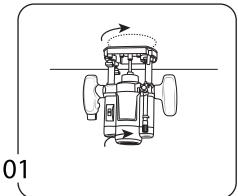
**STEP 1:** On the underside of the surface, machine a  $2.6^{\prime\prime}$  diameter recess to a depth leaving <  $0.1^{\prime\prime}$  of material.
